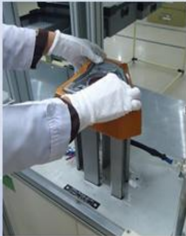
ANNEALED PART PLACED ON AIR LEAKAGE TEST JIG
